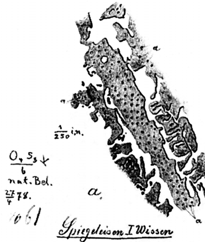
Metallographical sections of a steel specimen with "Spiegeleisen", Left hand of section normal to the cleavage surface, right hand parallel to it Martens, 1878
