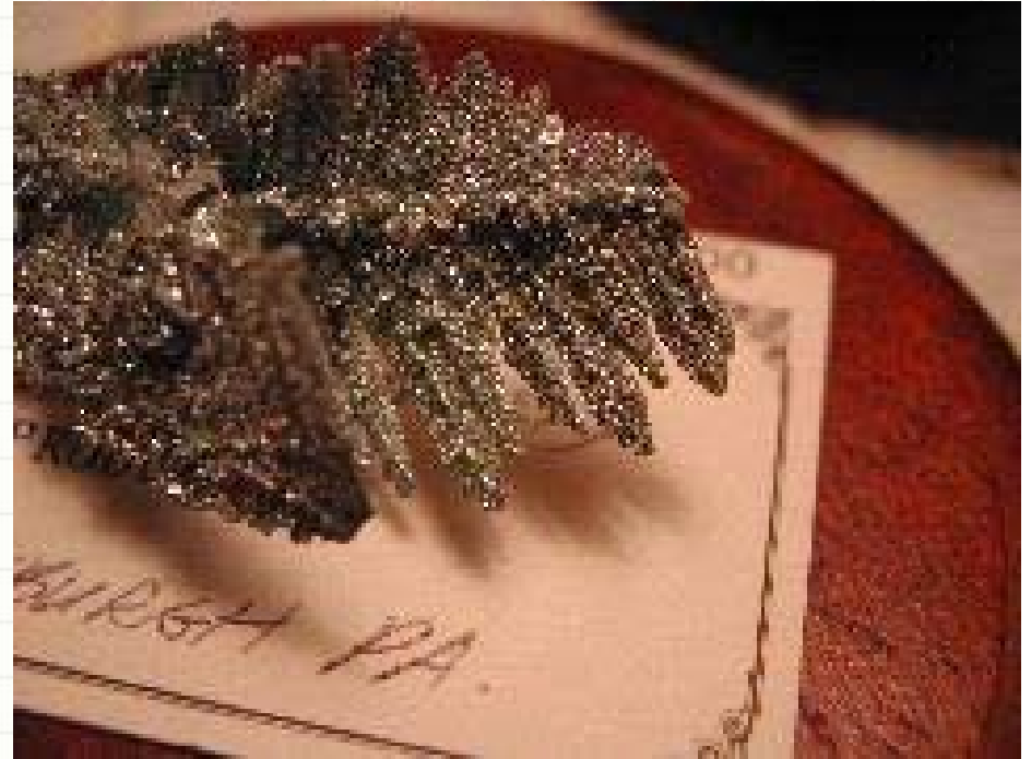
Dendrites of zinc rescued from partially solidified melt.
