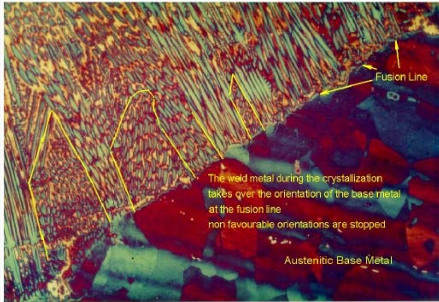
Crystallization of austenitic weld metal on the base metal
