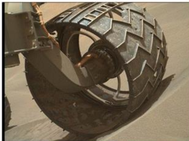
Figure 2. Curiosity's wheels showing signs of severe damage after almost 10 km of traverse.
