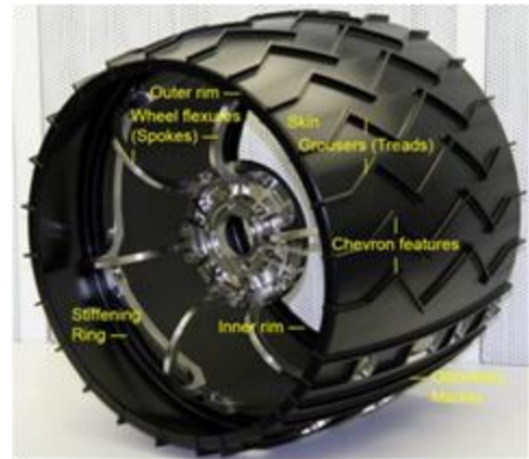
Figure 1. Curiosity's wheel made from a single piece of machined aluminum alloy AA7075-T7351. The main rim is 1.9 cm thick (0.75-inches). NASA / JPL / Emily Lakdawalla.
