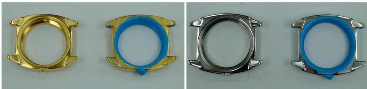
Nickel containing austenitic stainless-steel watch cases were submitted to the approved CEN nickel release tests, with nonsignificant surfaces masked as shown in accordance with the specified test method.
